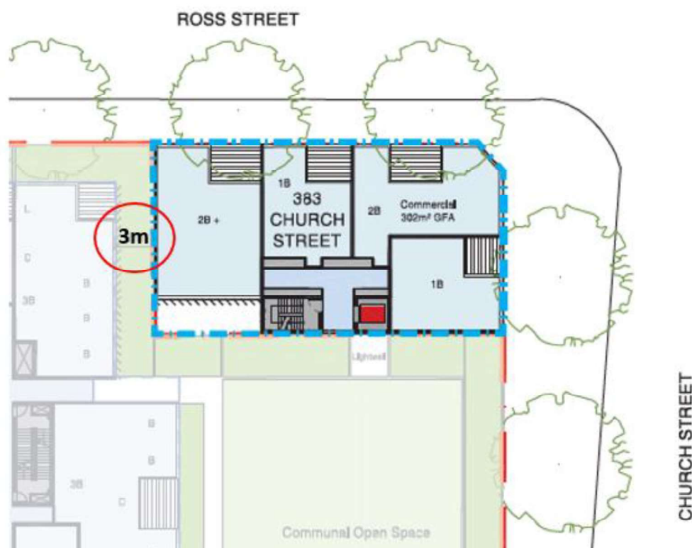
Figure 11: Illustration of upper level setback issue between reference design scheme and adjacent potential redevelopment of 383 Church St
